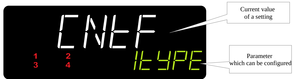
Fig. 10: View of menu when setting a parameter.
