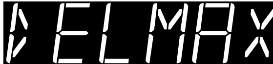
Fig. 13: The message after resetting the maximum value.
