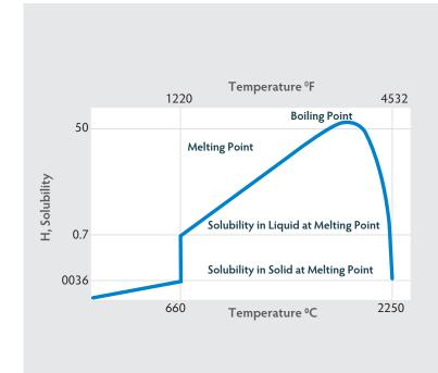
Hydrogen is the only gas that is appreciably soluble in molten aluminum and arises from the reaction between molten aluminum & water vapor (2Al +  $3H_2O = Al_2O3 + 3H_2$ ). As solubility of hydrogen in aluminum is significantly lower in the solid form than in molten, the dissolved hydrogen bubbles to the surface as the melt is solidified.
