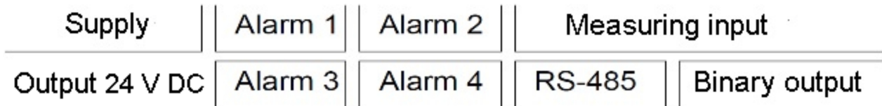
Fig. 4: Galvanic isolation of the N32U meter.
