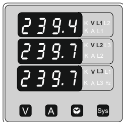
Screen 3 : Voltage Single Phase (For Single only)
