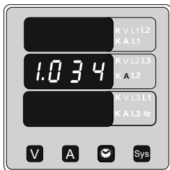
Screen 5 : Phase Current (For Single Phase only)
